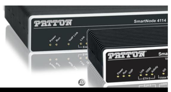
The SmartNode 4110 Series of VoIP Media Gateways supports up to eight telephone connections integrating PSTN, PBX, and standard phones for voice and fax over any IP network. Now the corporate, small, or remote office can use voice-over-packet services to eliminate toll charges, access local PSTN calling, and secure voice traffic end-to-end.
