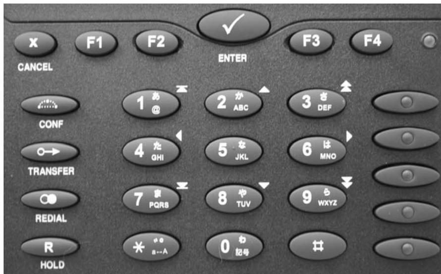
The MENU key **MENU** is used to invoke the main menu. To cancel actions or input, the CANCEL key **X** can be used. The ENTER key **✓** confirms actions, selections and inputs.
