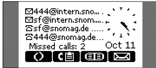
On the idle screen, the letter icon to the left of the SIP registration line indicates the registered phone number the call was recorded for. After you press the function key
