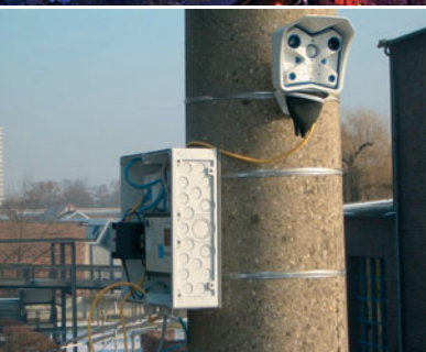
MOBOTIX camera with the Mobile Connect Box for the UMTS transmission of current traffic images (during installation still open).
