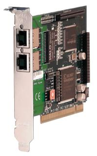
The TE205P and TE210P support industry standard telephony and data protocols, including Primary Rate ISDN (both N. American and Standard Euro) protocol families for voice, PPP, Cisco, HDLC, and Frame Relay data modes. Both line-side and trunk-side interfaces are supported, also included are advanced call features.
