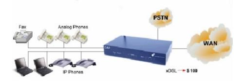
The CAP eliminates the need to install and maintain as many as five separate products. It integrates IP QoS, firewall, VPN, and more in an all-in-one platform that enables secure, SLAmanaged VoIP, IP videoconferencing and business IP services for SMB/SME and remote office customers.
