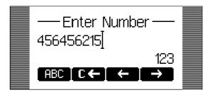
If block dial, the default setting, is on and the user has not pressed any keys for a few seconds, the phone will remind the user to press ENTER in order to start the call.
