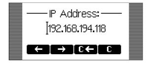
A valid IP address appropriate to the network in which the phone is being used can be provided.
