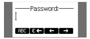
The default mode for password input is integer. You can switch to other input modes by pressing 123, ABC, or 3bc. The password is hidden and replaced by a series of \*s to keep it hidden from prying eyes.
