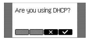
The phone has a built-in DHCP client. It will receive an IP address and other network-related settings (Netmask, IP gateway, DNS server) from the DHCP server.
