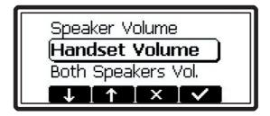
Here the volume of the casing speaker, of the handset speaker or of both can be adjusted. Select one of the three choices and you will see a display similar to the one below.
