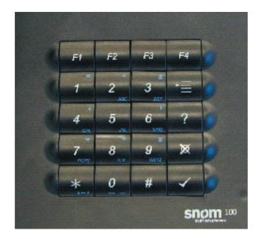
The MENU key 🔄 is used to invoke the main menu. The HELP key ? brings up context specific help texts. To cancel actions or input the CANCEL key 🛛 can be used. The Enter/Ok key 🗹 confirms actions, selections and inputs.
