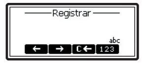
Type in the requested information and confirm with the enter key. The phone tries to register your given account name at the given registrar. The idle screen is shown and the first SIP line displays your registration.
