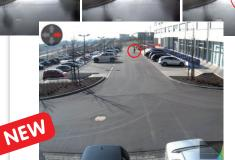
The MxActivitySensor is an activity-controlled, software-based image analysis function for detecting movement of people and objects in a monitored area (full image or section). Unlike existing video motion sensors, which detect all events in the defined motion windows, the MxActivitySensor is very easy to configure and delivers reliable results, even in applications with large amounts of external interference.
