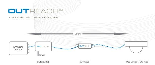
In this application, POE capability is added to the network connection using Veracity's OUTSOURCE power injector. OUTSOURCE not only upgrades the standard switch's Ethernet port to be POE compatible, but is able to deliver extra power to the OUTREACH, above the usual maximum for POE.
