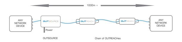
OUTREACH will also extend Ethernet without POE to all standard network devices, and the maximum extension distance is greatest when there is no requirement for POE to be forwarded. The example above shows an OUTSOURCE powering a chain of OUTREACHes
