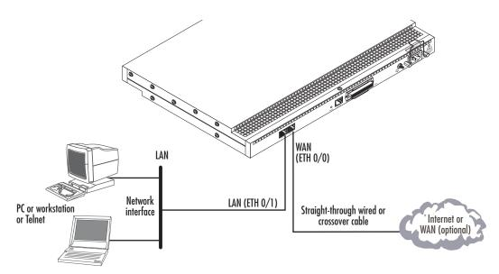
Figure 18. Connecting the SmartNode to the network
