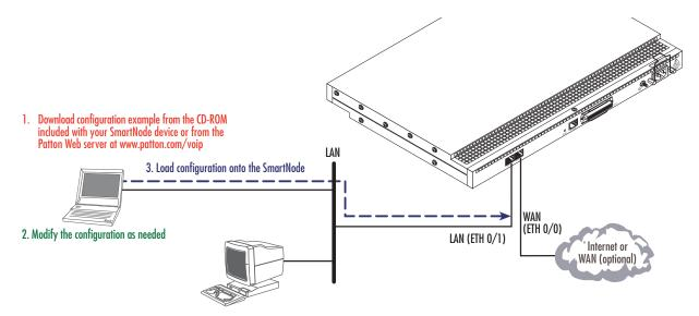
Figure 16. Loading the configuration
