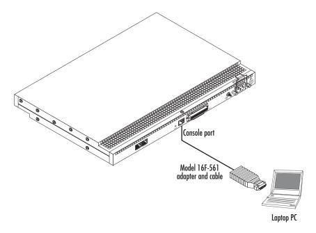
Figure 17. Connecting to the RS-232 Console port
