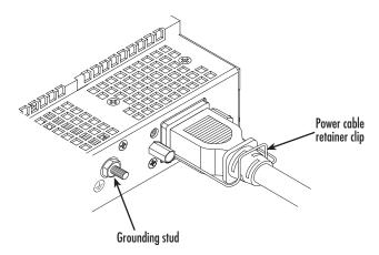
Figure 12. Grounding stud and power cable retainer clip
