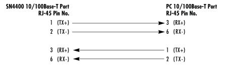
Figure 9. Cross-over RJ-45-to-RJ-45 Ethernet cable diagram
