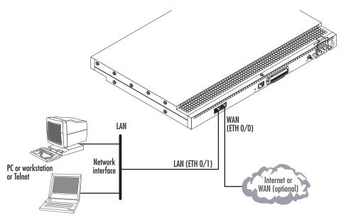
Figure 15. Connecting the SmartNode to the network
