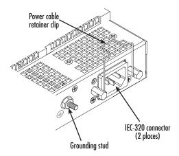
Figure 11. IEC-320 connector and grounding stud locations
