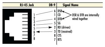
Figure 10. DB-9-to-RJ-45 cable diagram
