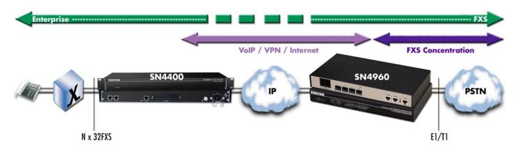
Figure 4. Enterprise FXS concentration and extension over IP and T1/E1
