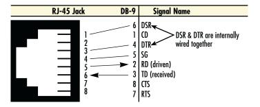
Figure 19. EIA-561 (RJ-45 8-pin) port
