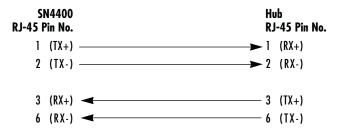
Figure 8. Straight-through RJ-45-to-RJ-45 Ethernet cable diagram
