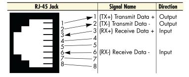
Figure 7. Model SN4400 Ethernet port
